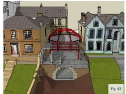
6) Ground floor external and internal walls constructed, brick work to basement built up and steel dome structure erected
