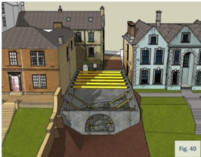
4) Horizontal support props installed so raking props can be removed for basement floor slab to be cast
