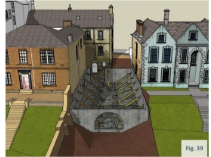
3) Basement walls completed. Raking support props installed to provide lateral support against thrust of existing foundations
